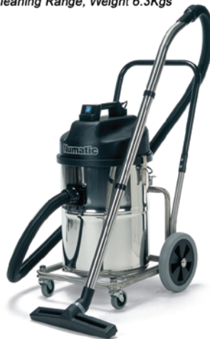
WV750F-2 35L/25L Wet & Dry Commercial Vacuum Cleaner, 1200W, 38mm BB8 Kit, 35 Litre Dry Capacity, 25 Litre Wet Capacity, 26.8m Cleaning Range, Fixed Chassis, H 940mm.
